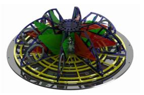
8 sectors with 24 antennas Frequency range: 9kHz to 6 / 20 / 40GHz
